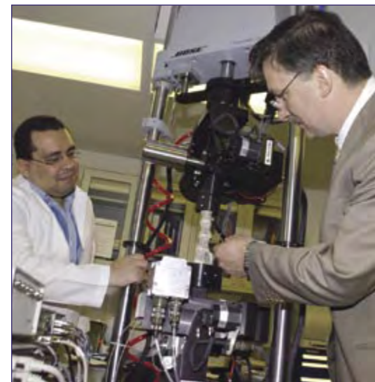
Tariq E. Awad, MD, and lab co-director director William C. Welch, MD, examine a lumbar spine specimen as the Bose Spine Tester performs flexion/extension testing.
